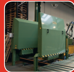
Different pallet lengths - Adaptation of the sides
